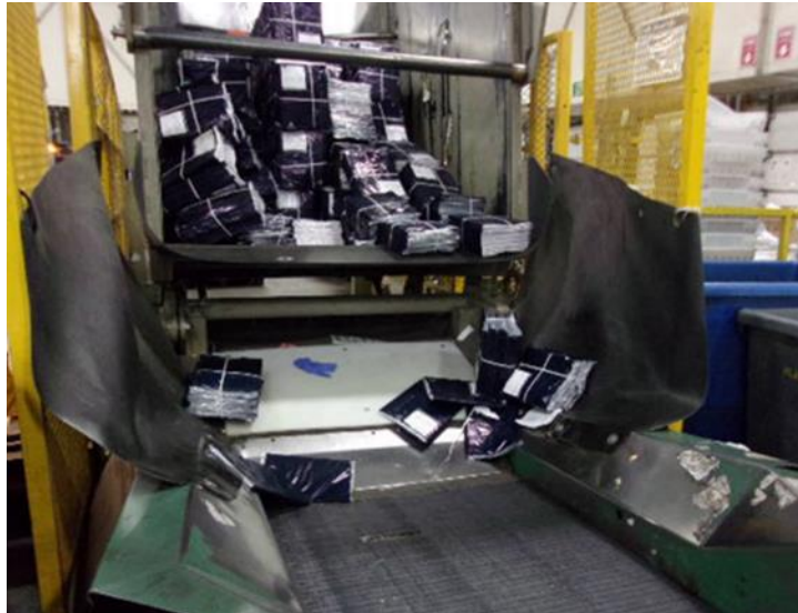
Picture III-1 APBS—Bundles Inducted From the Dumper Onto a Conveyor Belt
