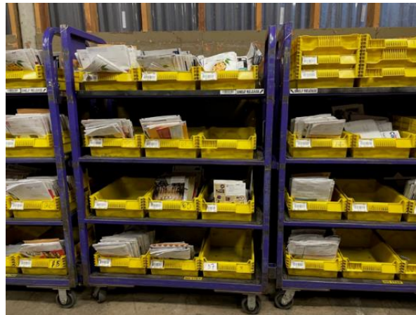
Picture III-14 Flats That Arrived from an Upstream P&DC Sorted to DPS
