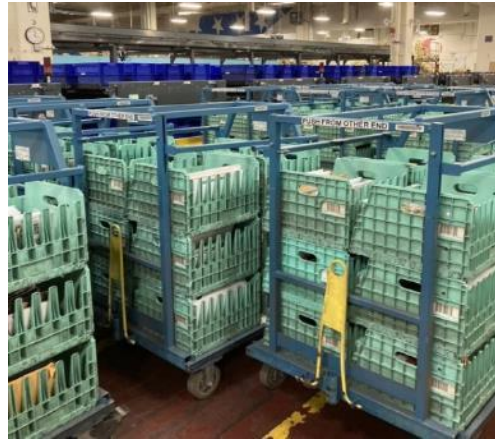
Picture III-6 Flats in Trays Compatible with FSS Are Gathered for Sorting on FSS Equipment
