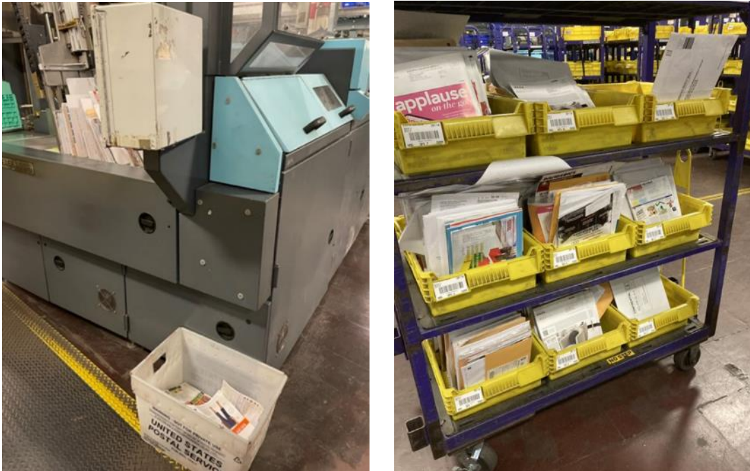
(Left: Bin with pieces that fell out or got jammed during FSS machine run. Right: “No-read” rejects from FSS)
